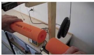
Cut the pool noodle twice on the markings, you can use an electric carving knife, razor blade or a hot wire.
