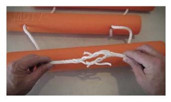
Push the ropes together so that the strands on the right alternate between the strands on the left.
