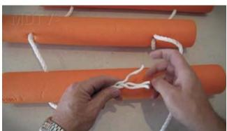
Untwist a section of each rope, back to the point where the ropes met (as determined 2 steps ago)
