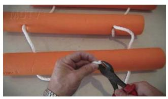
If the ends of the rope are melted together, you will need to cut the strands loose on both ends
