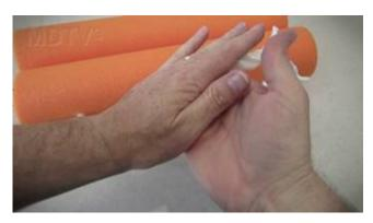
Roll the spliced rope between your hands a few times to fully seat it into position.
