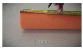
Mark out the positions of the holes, 100mm in from each end on all sections
