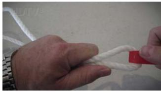
Fold the rope in half and mark the center of the rope with tape
