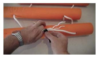
Hold one side of the strands and the rope together and tape off the other side of rope and strands
