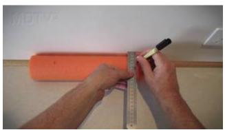
To make sure the holes are in the same line you can place the sections against a wall and measure out the same distance from the wall.
