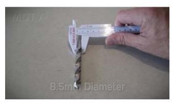
Use a drill bigger than the rope diameter; I'm using an 8.5mm drill.
