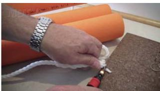
Cut the excess off with a hot knife or heated blade for best results.
